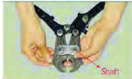
Step1:Installing jaw on to the tool
